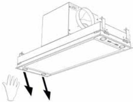
2. Removing the LED lamp:
